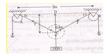
Q5.) Find the forces on a bolt as shown in the below fig. Determine the resultant of forces on the bolt.
