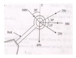
Q6.) Determine the resultant and equilibrant of the forces acting as shown in the below fig.
